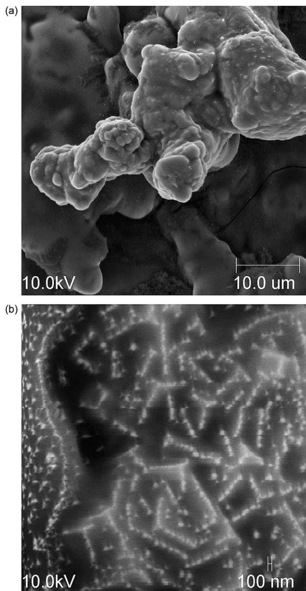
Fig. 2. SEM micrographs of the (a) surface ( $\times 1500$ ) and (b) cross-section ( $\times 3000$ ) of a PPy/PCPS composite.
