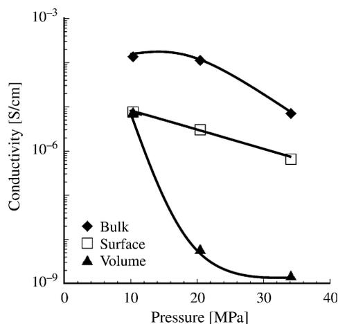
Fig. 5. Electrical conductivity of PPy/PCPS composites at 313 K as a function of  $\text{CO}_2$  pressure.
