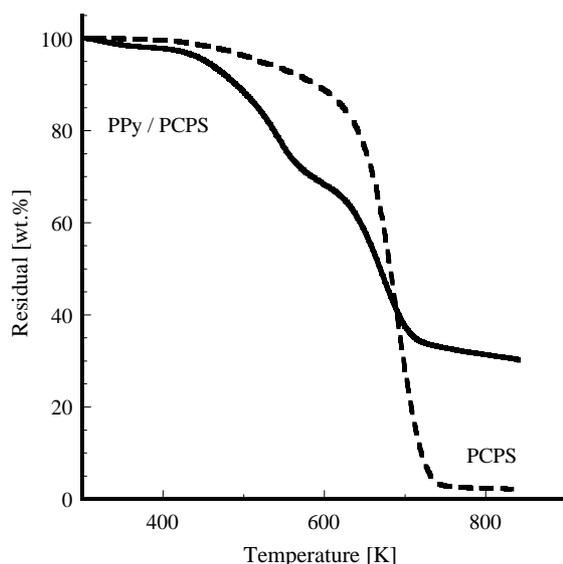
Fig. 6. Thermogravimetric analysis of PCPS and its composite with PPy.
