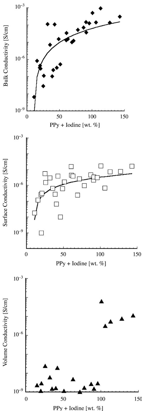
Fig. 4. Bulk, surface, and volume conductivities of PPy/PCPS composites.
