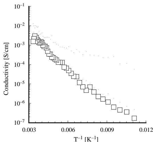
Fig. 8. Arrhenius plot of conductivity.
