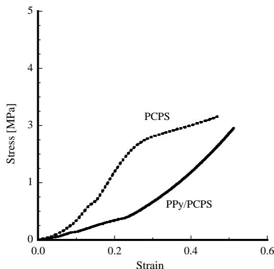
Fig. 7. Compressive stress–strain curve of PCPS and its composite with PPy.
