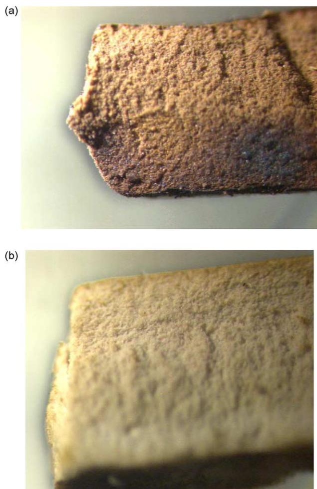
Fig. 1. Optical micrographs of the cross-section of the (a) exposed and (b) unexposed surfaces of a PCPS sample exposed to  $I_2$  vapor ( $\times 25$ ).
