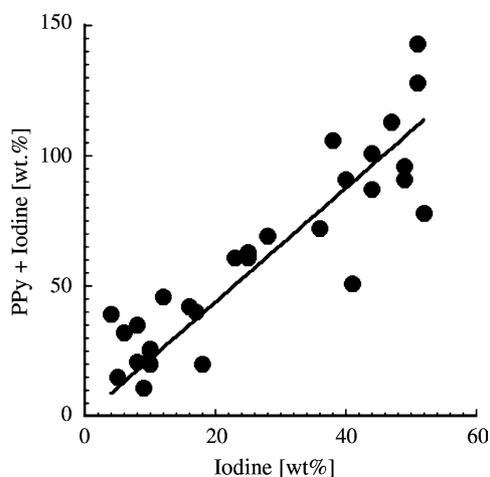
Fig. 3. Amount of conductive PPy + I<sub>2</sub> complex in the PPy/PCPS composite as a function of amount of I<sub>2</sub> impregnated.
